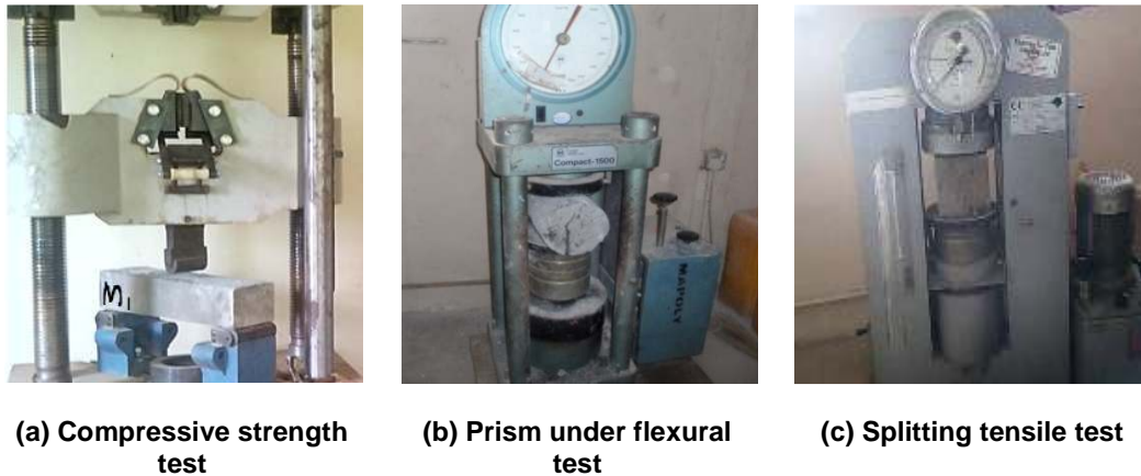
Fig. 5. Strength characteristics tests set-up of specimens
