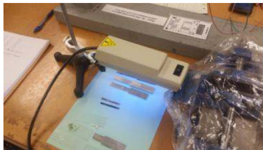
Fig. 1. UV light excited photodecomposition test set-up
