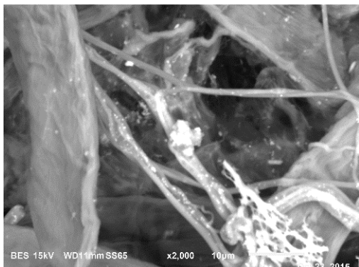
Fig. 12. SEM image showing the exposure of nanoparticles from the electrospun fibers
